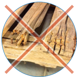
Cracks on the top or bottom boards greater than 1/8" W x 15" L are NOT ALLOWED .
