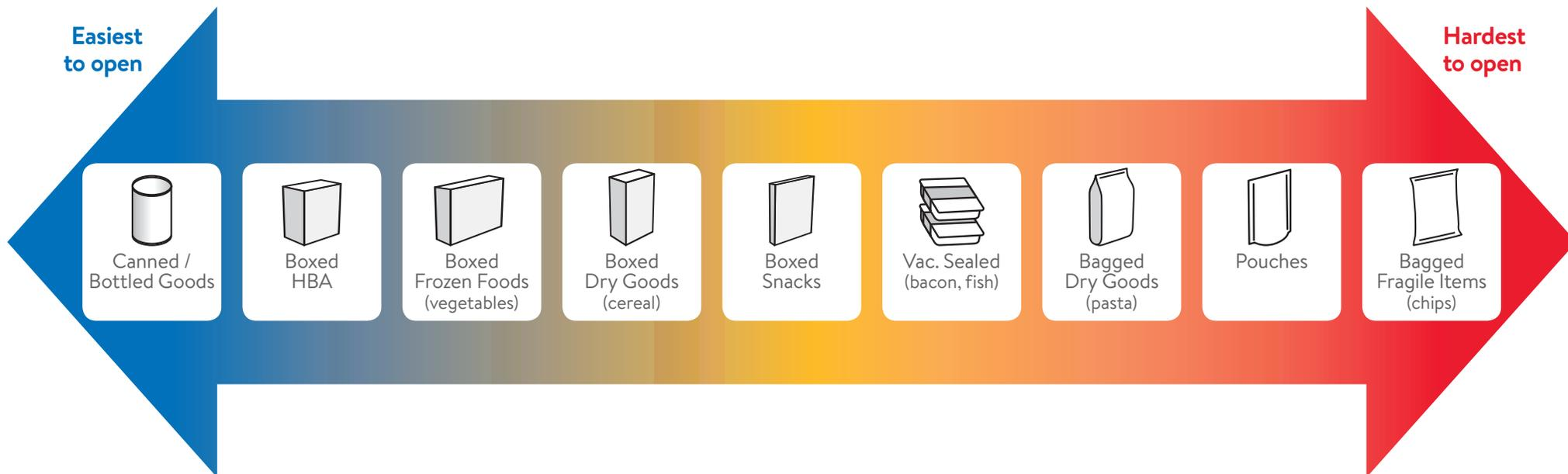
The product inside an SRP can help or hinder the structural strength of a box. Oftentimes the stacking strength of a box can be enhanced or weakened by the product inside as much as any other single factor. For example, a box, SRP, or tray with canned products will get significantly more stacking strength from the cans, while a box of chips requires that 100% of its stacking strength come from the box.
