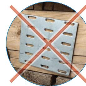
No double stringers, patched boards or metal repair plates
